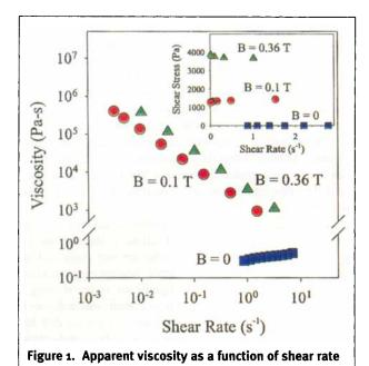
for an MR fluid composed of carbonyl iron particles (50 µm dia) in silicone oil (10 vol %) for different applied magnetic field strengths (Rankin et al., 1999; Rankin, 2000).
