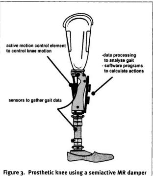
Figure 3. Prosthetic knee using a semiactive MR damper (Carlson and Sproston, 2000).
